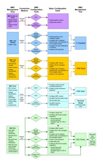
Figure 1-1. BMC Configuration Matrix
