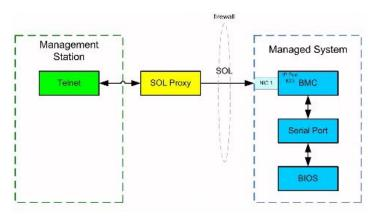
Figure 3-15. SOL Proxy Diagram
